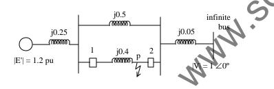
Find the critical clearing angle for clearing the fault with simultaneous opening of the breakers 1 and 2. The reactance values of various components are indicated on diagram. The generator is delivering 1.0 pu power at the instant preceding the fault. 7
